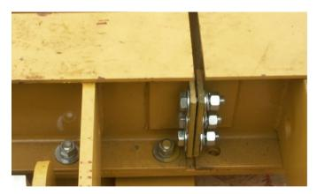
8. Bolt the bulkheads to each end of the scale. Using four 3/4" x 2-1/4" bolts per end.
