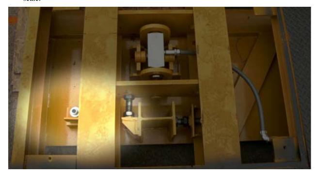
11. Adjust the Bumper bolts to minimum of 1/8" and a maximum of 1/4" on all four corners of the scale sections. Total of eight bumpers per section.
