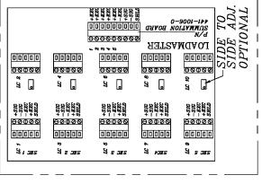
MAIN CABLE FROM SCALES TO SECTION ADJUST L 03 #8778 WIRE COLORS BLK/CRN PAIR USE GRN +EXC SEC BLK/YEL PAIR USE YEL +EXC SEC BELDON CABLE
